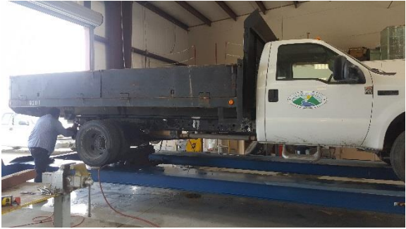
Shop retro-fit the dump bed from old truck (CARB) to used tool truck.
