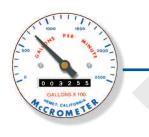
The McCrometer Propeller flowmeter comes with a standard instantaneous flowrate indicator and straight-reading totalizer. An optional electronic FlowCom register is also available.
