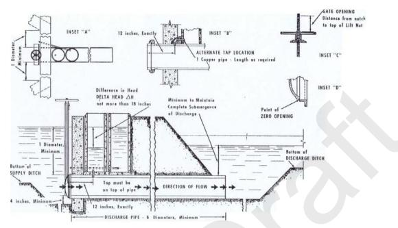
Figure 1. Metergate drawing used by various manufacturers, USBR, etc.
