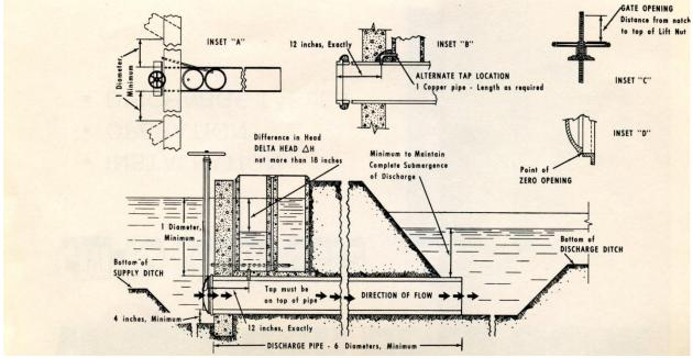
Figure 1. Typical Tulare Irrigation District Meter Gate Installation
