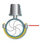
The positioning of the impeller directly in the flow stream assures full-flow measurement and greater accuracy.
