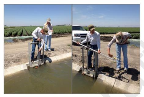
Figure 5. Special tool to detect actual gate opening.
