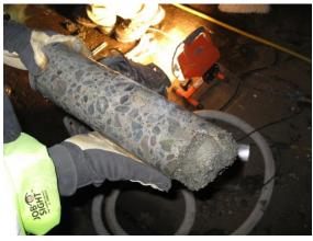
Main Intake Canal Siphon coring sample.
