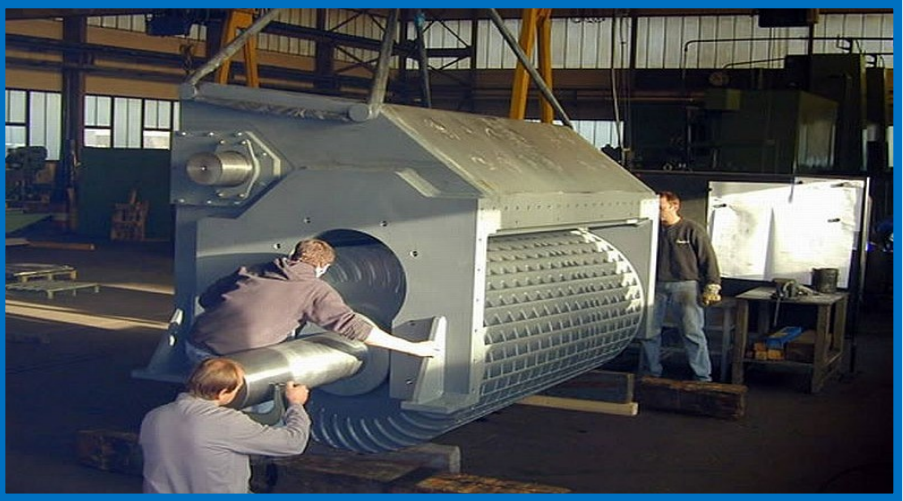
Cross-Flow Turbine - Under Consideration by Kaweah River Power Authority
